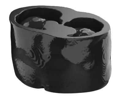
This abdomen phantom can be used in CT for image quality evaluation and for training. It was also designed to enable evaluation of diagnostic software, including AI tools.
