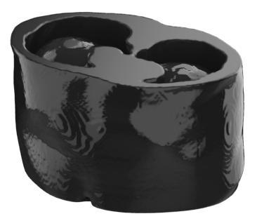
This abdomen phantom can be used in CT for evaluation of low-contrast lesions in the pancreas. It was designed to enable evaluation of diagnostic software, including Al tools.
