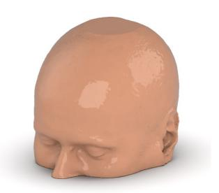
This phantom simulates a contrast medium enhanced head in arterial phase (CT angiography). The neck is included up to the first cervical vertebra. The vertex is included until approximately 0.5 cm below skin level.
